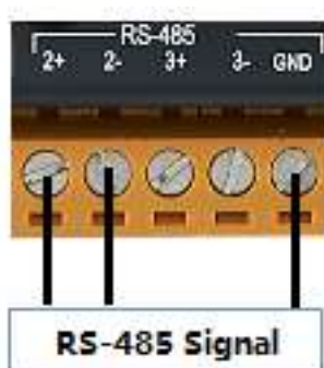
Figure 3.5 Serial Port Wiring
