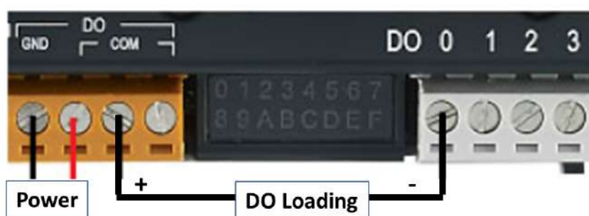
Figure 3.4 Digital Output Wiring
