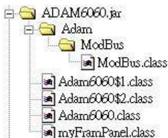
Figure 5.25: Structure of the ADAM6060.jar file
