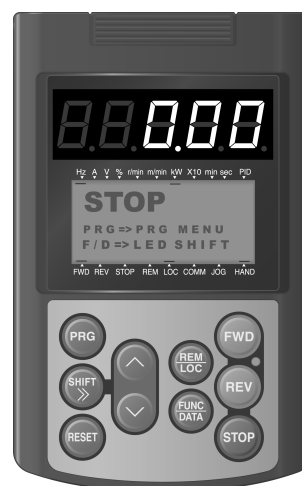
Figure 4.3 Indication on LED Monitor and LCD monitor after Power-on
